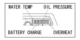
Under normal condition, when the starter switch changes from STOP to RUN, all the lamps of BATTERY CHARGING, OIL PRESSURE and Hz/OVERHEAT turn ON. When the engine starts, all the lamps turn OFF. When abnormality is detected on other than Hz/OVERHEAT, the corresponding monitor lamp will flash, and the engine automatically shutoff.
